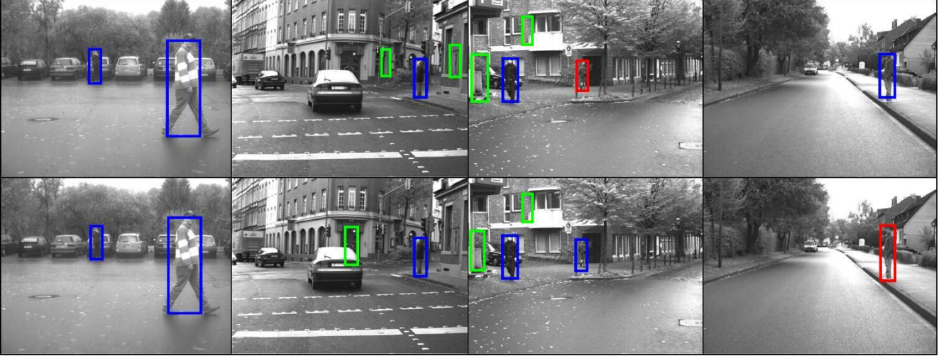
Figure 5. Qualitative results at 10^0 FPPI taken when following Daimler criteria. Top row: using the pedestrian detector based on Daimler’s training set. Bottom row: using the pedestrian detector corresponding to the training with virtual samples, in particular with the classifier of highest detection rate at 10^0 FPPI. Blue bounding boxes are right detections, green ones are false positives and red ones misdetections.
