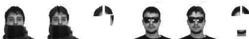
Fig. 1. Example of face images from the AR Face database [14] where different fragments are analyzed at each position. The first image shows the original face, in the second image we plot only the 5 most similar fragments according to the normalized correlation on the face. The third image shows the fragments alone.
