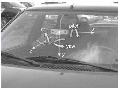
Fig. 1 On-board stereo vision sensor with co-ordinate system
