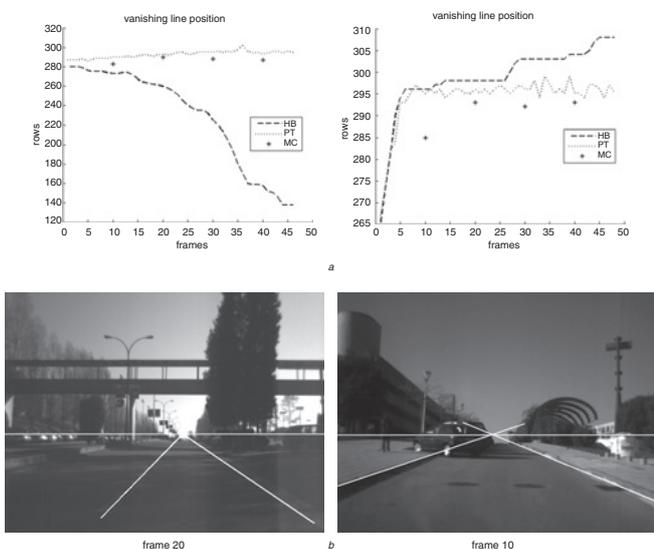
Fig. 3 Illustrations of two different scenarios: flat road and uphill driving
