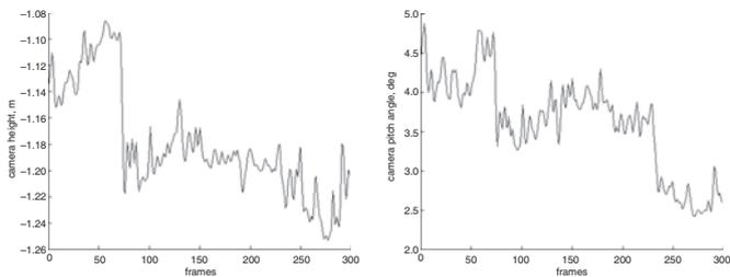
Fig. 2 Estimated camera height and pitch angle against time, related to current fitted plane (only 2 fps plotted)
