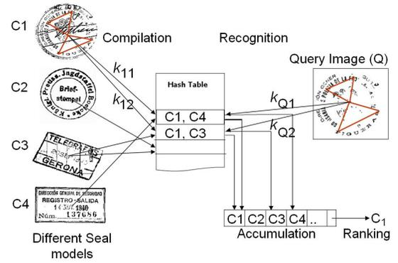
**Figure 6. Model generation and Seal recognition architecture**
