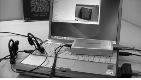
**Figure 1. Wearable Camera System.**
