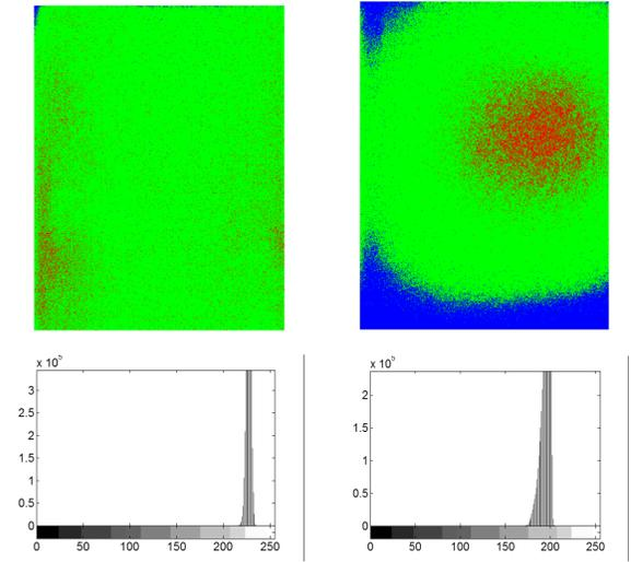
**Figure 5. Left: Gray level contours for a uniformly colored document taken with the Epson Perfection 3170 Photo scanner. The highlighted levels are <220 (blue), 220-230 (green), >230 (red); Right: Gray level contours for the same document taken with the Canon camera. The highlighted levels are <190 (blue), 190-200 (green), >200 (red).**
