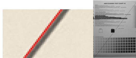
**Figure 2. Geometric Linearity of the Canon G10 with an AIIM Scanner Test Chart #2. The red line segment is superimposed on bitmap.**
