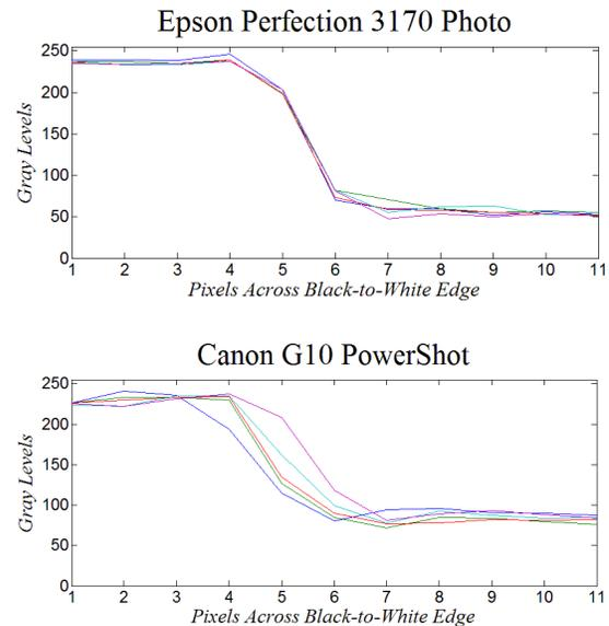
**Figure 3. Edge step response of scanner and camera at 262 dpi at five different locations of a sharp white-to-black edge on an AIIM Scanner Test Chart #2.**
