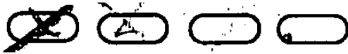
Figure 2. Example of a recognition result: the race’s ground-truth is VNNN (Vote, No-Vote, No-Vote, No-Vote). The native Ex recognizer reads it correctly as VNNN, the Check recognizer reads it as VVNN, the Filled recognizer reads it as NNNN, the Blend recognizer reads it as VVNN, and the Separate recognizer reads it as VVNN. The style-based recognizer reads it correctly as VNNN.
