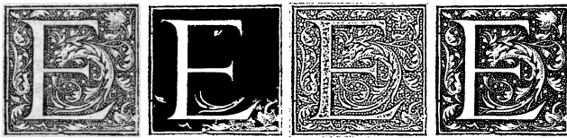
Figure 3. From left to right: original drop cap, binarization using the proposed method (M1), method of Trier and Taxt (M2) and method based on fuzzy entropy (M3).
