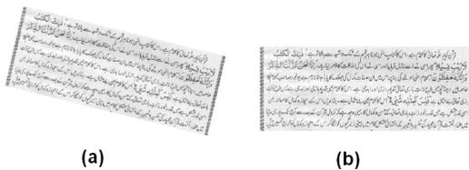
**Figure 6. (a) Original skewed image (Arabic mixed with Urdu), (b) Skew corrected image by our algorithm**
