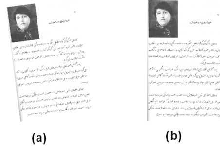
**Figure 7. (a) Original skewed image (Farsi), (b) Skew corrected image by our algorithm**
