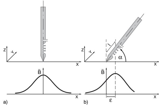
**Figure 2. The established magnetic field  $\vec{B}$  varies, depending on the pen's construction, its aerial characteristic and inclination. (a) With a perpendicular pen position the magnetic field  $\vec{B}$  is symmetric. (b) In contrast, with a pen tilt  $\alpha$  the magnetic field  $\vec{B}$  is skewed, which leads to a displacement  $\varepsilon$  of the maximal activation [9].**
