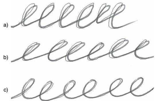
**Figure 1. Simultaneously produced on- and offline handwriting samples: (a) pen tilt  $< 45^\circ$ , (b) pen tilt  $\approx 55^\circ$  and (c) pen tilt  $\approx 90^\circ$ . Due to a tablet displacement error and a varying pen tilt, on- and offline handwriting samples do not match.**
