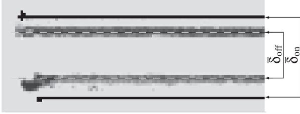
**Figure 3. Superimposed on- and offline traces produced simultaneously. Note that cross-coupling between pen tilt and pen-position activation has resulted in a systematic displacement error between on- and offline traces.**
