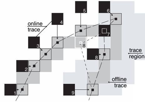
**Figure 4. Schematic overview of the superpositioning of on- and offline specimens. A general alignment of the on- and offline strokes is followed by the constrained morphing of online sample points to the nearest offline trace element of the assigned region.**
