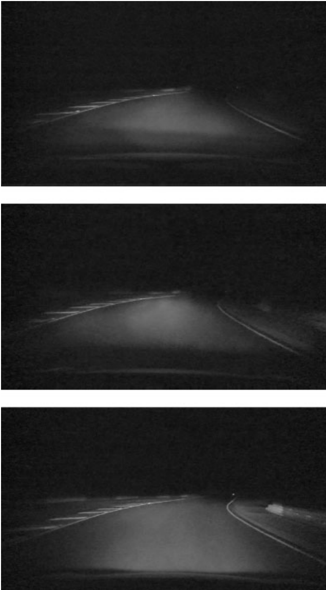
Fig. 1 Sample frames from different headlights: from top to bottom, Seat Ibiza simple headlamps, Seat Altea double headlamps and Seat Toledo AFS
