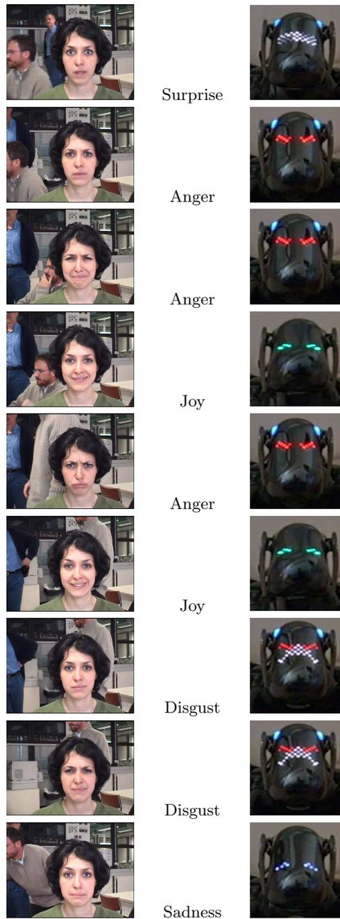
**Fig. 4.** **Left column:** Some detected keyframes associated with the 1600-frame original video. **Middle column:** The recognized expression. **Right column:** The corresponding robot's response.
