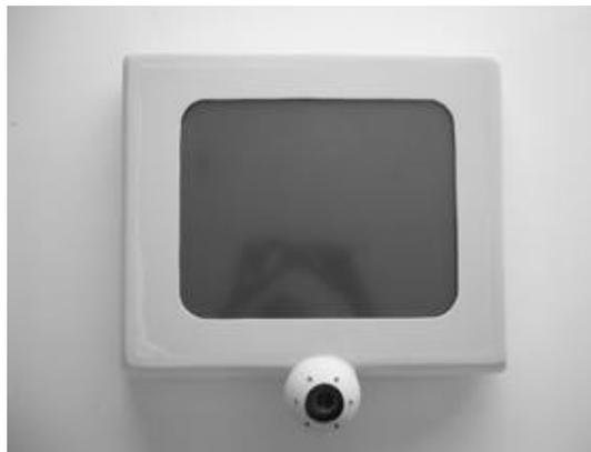
**Fig. 3.** A "transparent" representation for an ubiquitous computing component: a touchscreen enhanced with perceptive capability due to the embedded webcam
