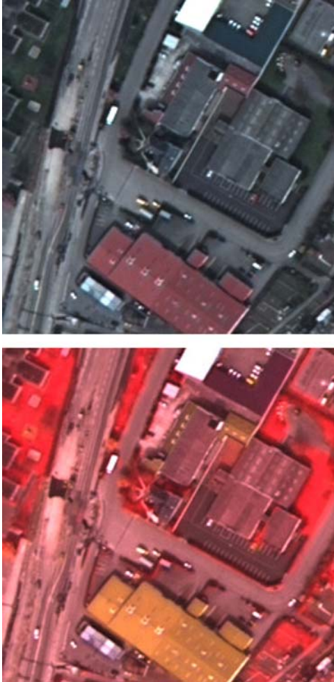
Figure 13. (a) Top: (R, G, B) channels of the reconstructed image obtained by interpolating the chromatic channels in the CIELAB color system. (b) Bottom: (IR, R, G) channels of the reconstructed image with the same method.
