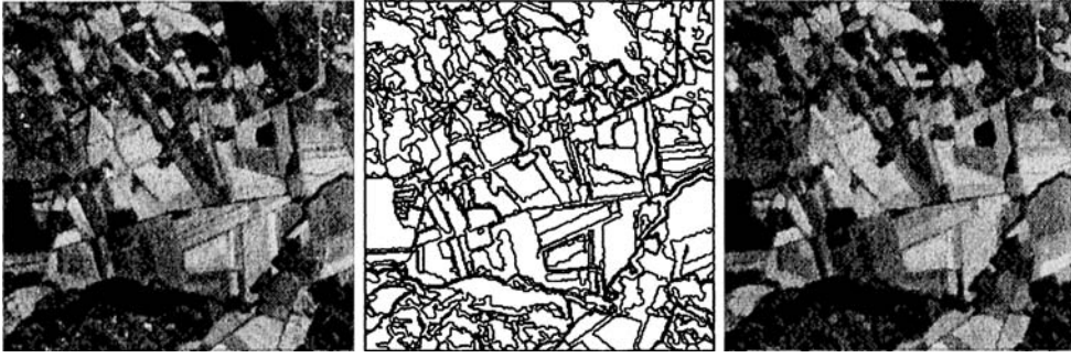
Figure 5. Result obtained minimizing E_{MS}^\lambda with \lambda = 200 using the algorithm described in Section 4. (a) Left: Original image, (b) Middle: Segmentation boundaries, (c) Right: the image \tilde{u} .
