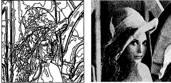
Figure 12. Experiment obtained minimizing (16) with \delta = 7 . (a) Left: the selected family of level lines. (b) Right: the function u_7 .
