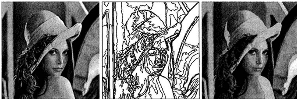
Figure 3. Result obtained minimizing E_{MS}^\lambda with \lambda = 100 using the algorithm described in Section 4. (a) Left: Original image, (b) Middle: Segmentation boundaries, (c) Right: the image \tilde{u} .
