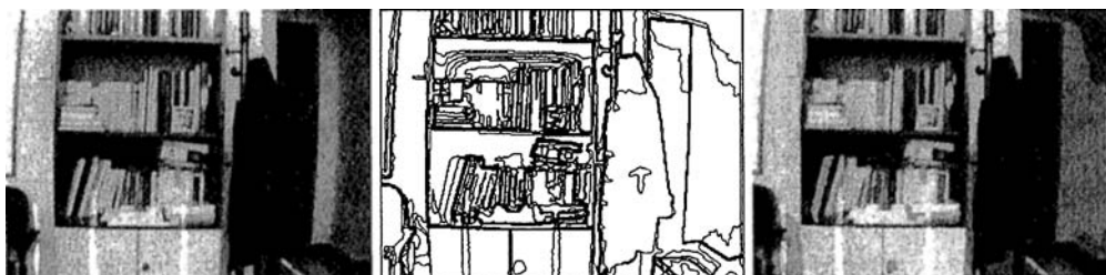
Figure 4. Result obtained minimizing E_{MS}^\lambda with \lambda = 60 using the algorithm described in Section 4. (a) Left: Original image, (b) Middle: Segmentation boundaries, (c) Right: the image \tilde{u} .
