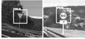
Figure 2: Detected traffic signs.
