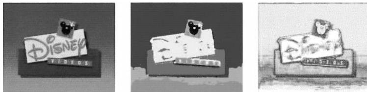
Figure 3. Meaning of the label probability maps seen in the case of a color gradient. The original image (left), its labeling using supervised training (middle) and the probabilities of this labeling (right) are shown (see color page – p. 271)
