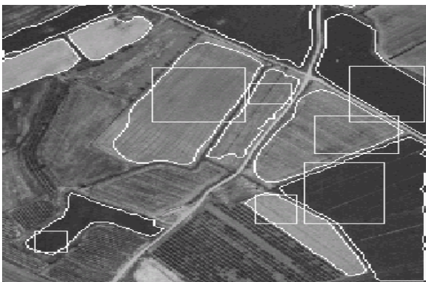
Figure 5. Seeds and boundaries result obtained 60% faster than manual drawn and with a sub-pixel accuracy.
